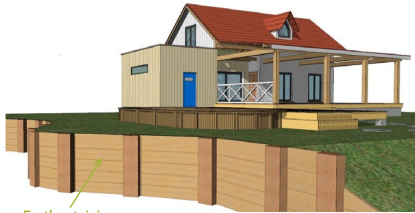
Earth retaining structure (4)
