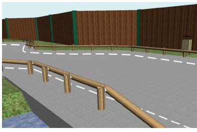
NB: The majority of these works should be considered to be in class 4 due to the complexity of their design. In all cases, the assembly of the components of the structure should allow for effective water drainage.
